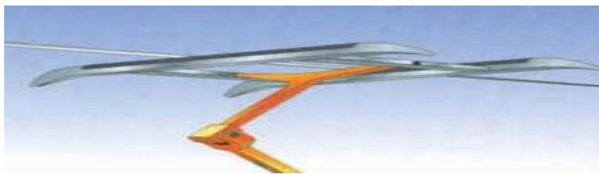
Figure 6: Sliding of the contact strip against contact wire.
