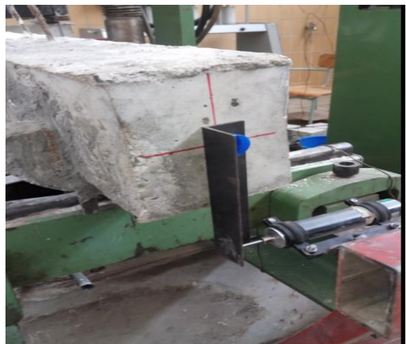
Figure 4-15-Angle of twist measurement using displacement transducer
