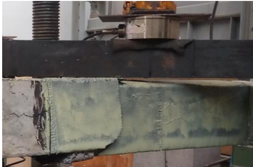
Figure 6-14- Rupture of the carbon fibers of specimen T100, 2
