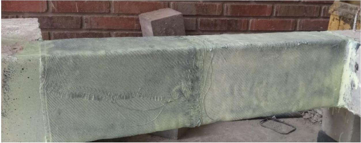
Figure 4-14- Specimen after the application of externally bonded carbon fibers
