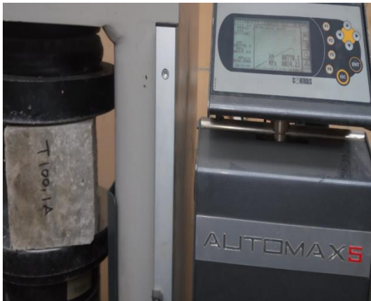
Figure 4-6- Compressive strength test
