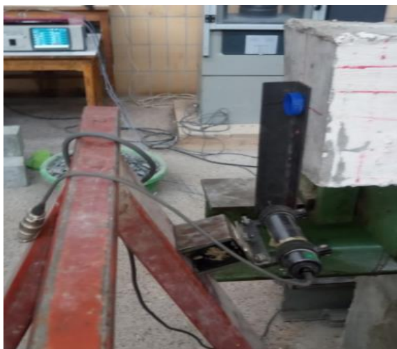
Figure 4-15-Angle of twist measurement using displacement transducer
