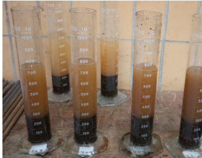
Figure 4-4- (a) Packed aggregates (b) Moisture content test (C) Silt content test
