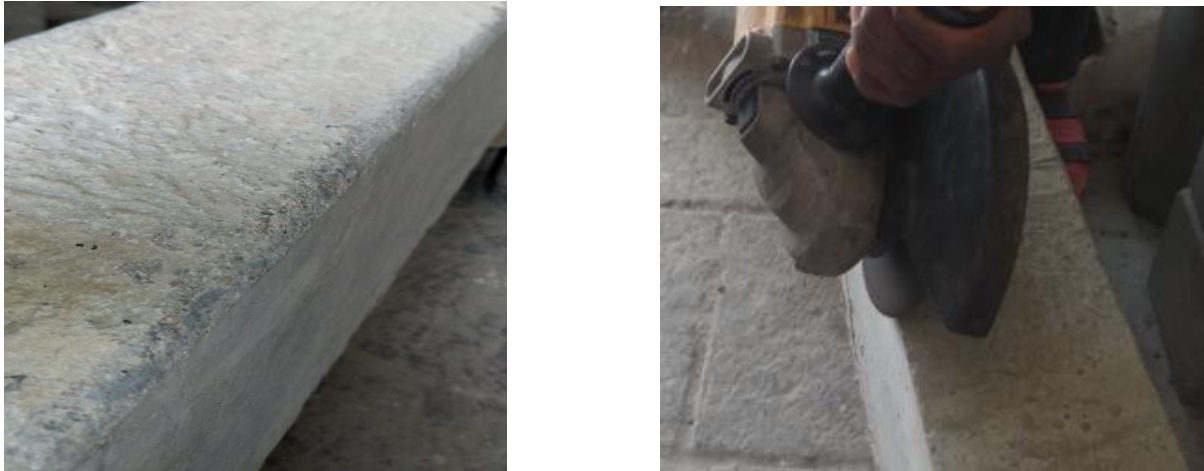
Figure 4-12- Specimen surface preparation
