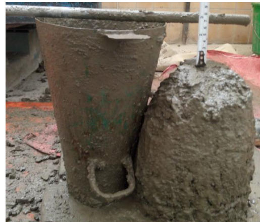
Figure 4-5- Concrete slump test
