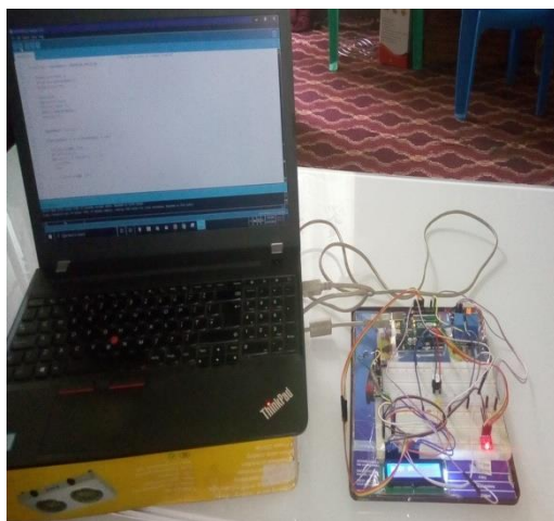
Figure 4.8: On Breadboard a SpO 2 sensing module
