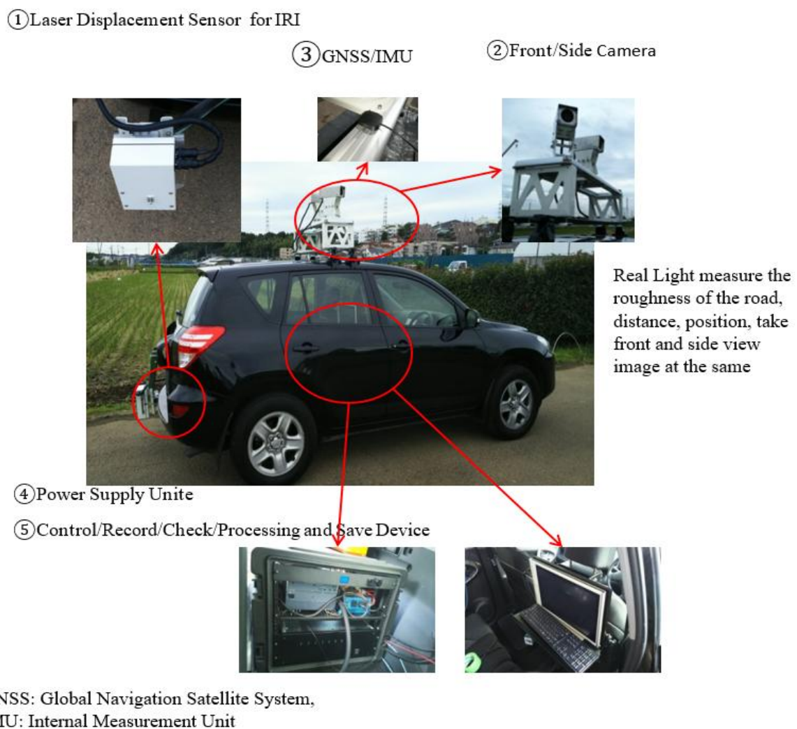
Figure 2-6: External and internal parts of the Pavement Condition Survey Vehicle
