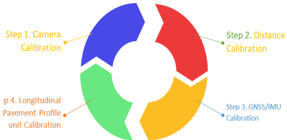
Figure 2-8: Pavement Condition Survey Vehicle PCSV Calibration process
