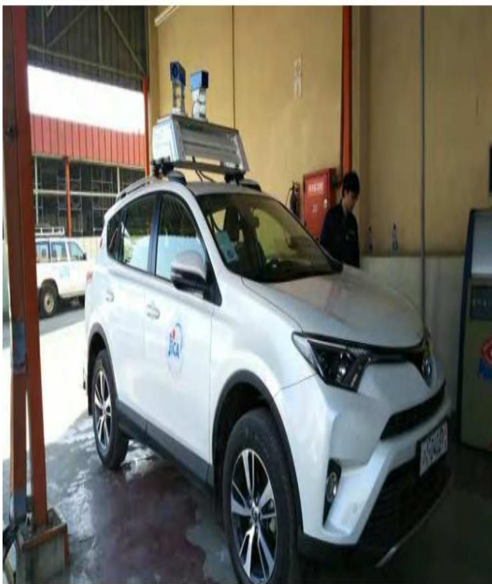
Figure 2-8: Pavement Condition Survey Vehicle PCSV Calibration process
