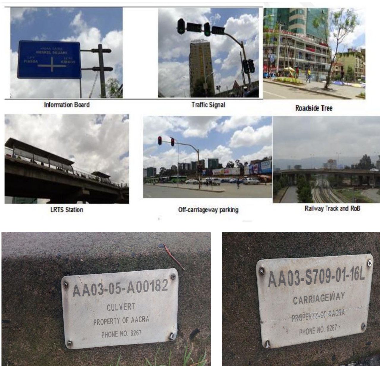
Figure 2 -14: AACRA's Traditional Road Infrastructure Asset Registration
