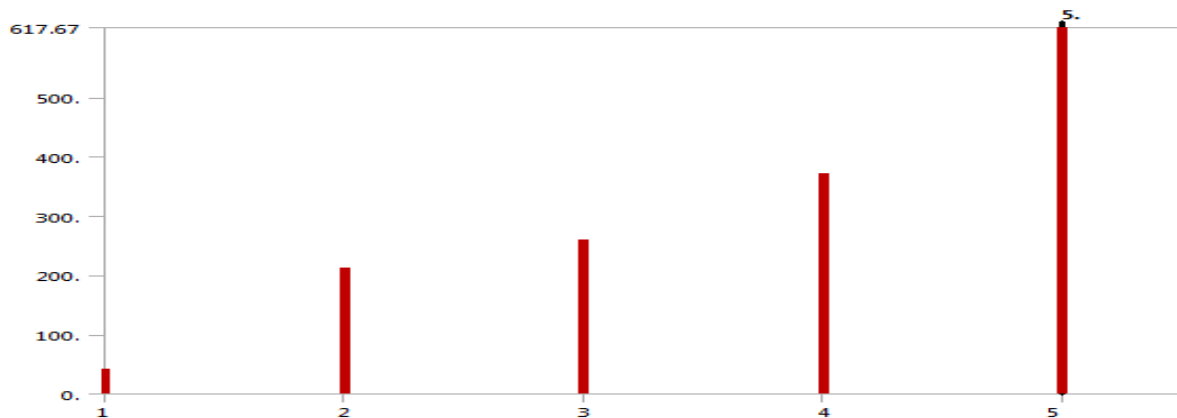
Fig.-16(h): The first five natural frequencies Vs. mode shape graph for a continuous rail
