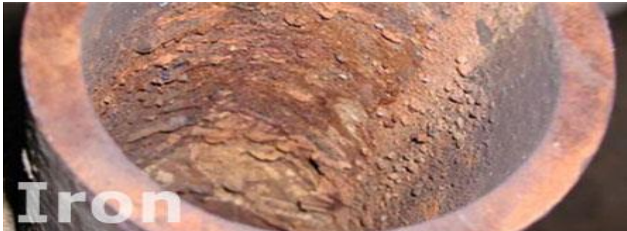
Figure 3 Impact of high level Iron on Pipe Material.
