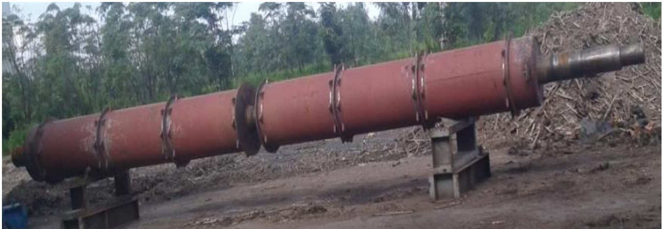
Figure 1.1: Existing feeder table head shaft in wonji-shoa sugar factory
