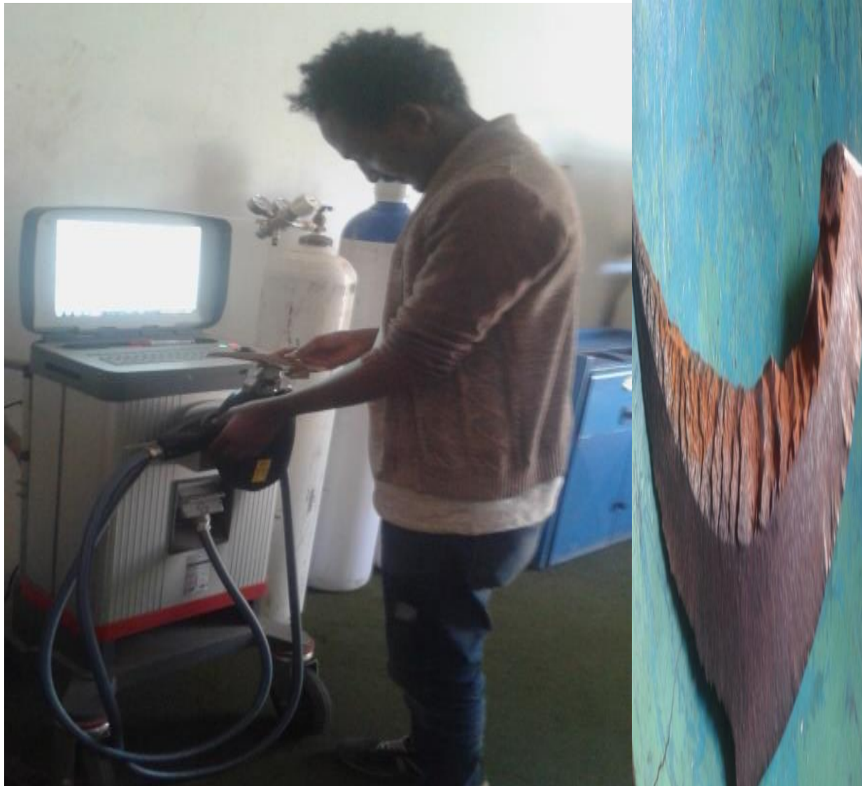
Figure 3.2: measuring composition material of the spacemen using Spectro test
