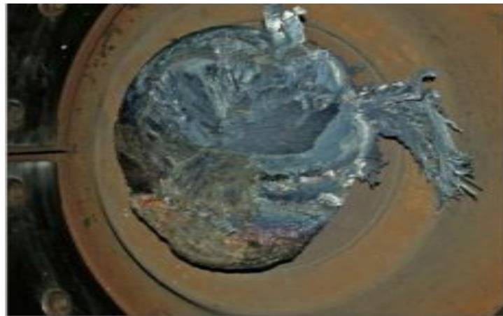
Fig 2.2 Fractured surface of an axle [11]
