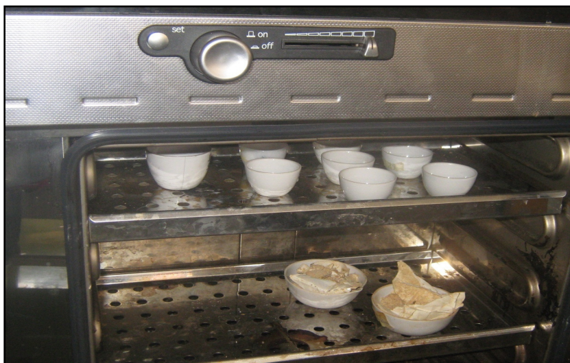
Figure 3.4: Wastewater samples in the oven for total solid analysis.
