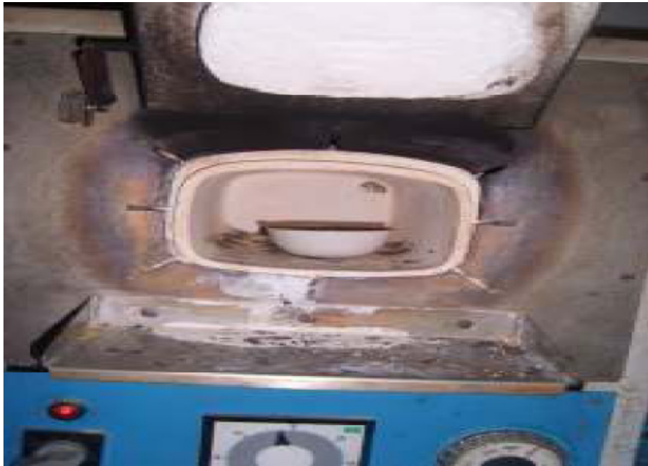
Figure 3.5: Wastewater samples in muffle furnace for volatile solid analysis.
