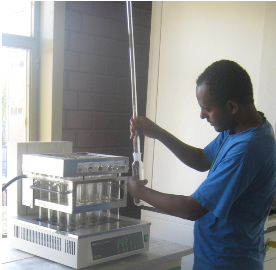
Figure 3.1: Wastewater sample analysis for COD determination.
