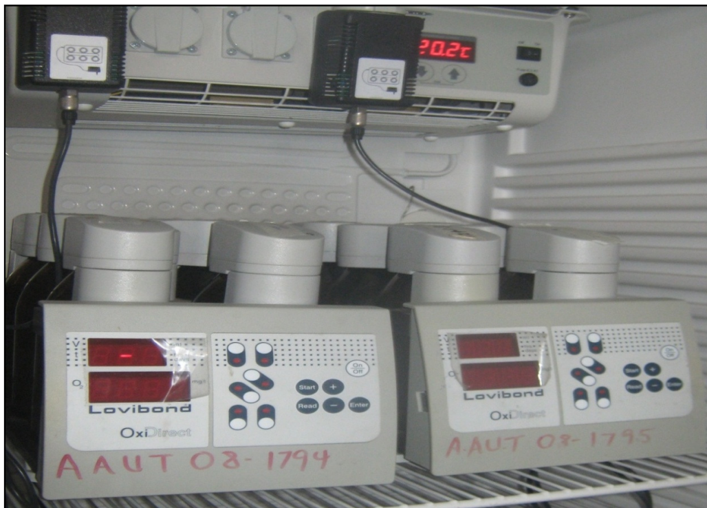
Figure 3.3: Wastewater samples in BOD 5 incubator.
