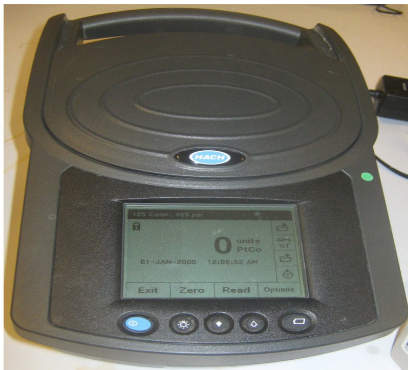
Figure 3.2: Spectrophotometer (HACH model) used for determination of the color of wastewater.
