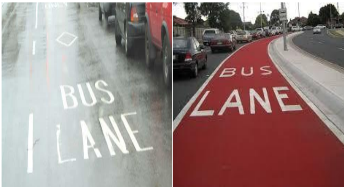
Figure 2.2: Line-separated Bus lane designs Groff, M. (2019).
