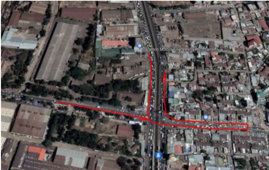
Figure 4-13: Possible routes for restricted Traffic (U-turn from west and North approaches and Left Turns from West approaches)
