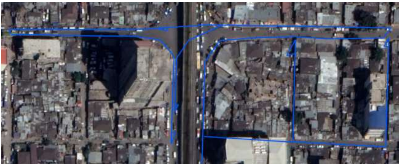
Figure 4-7: Possible Route option for U-Turn Restricted from Abinat Approaches. Unlike North south approaches, the East –West approaches are opened and possible to facilitate U-turn before the traffic inter to the intersection.
