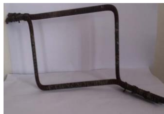
Figure 2-1 images showing assembled space swimmer bars loop (Moayyad Al-Nasra, 2017)
