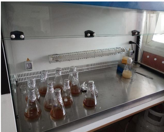
Pic G.9. Mixing of hydrolysate and inoculum
