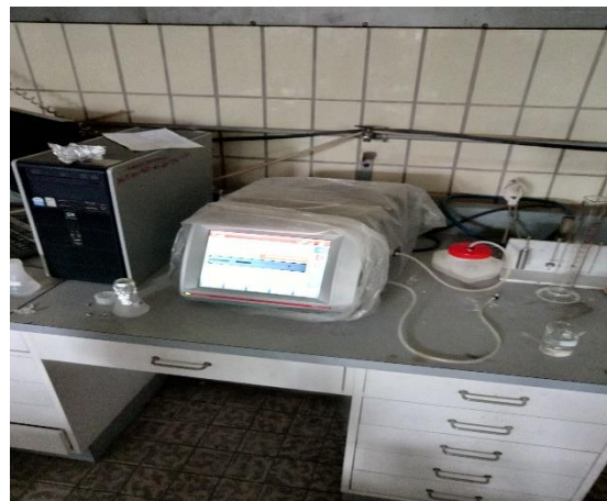
Pic G.10. Measuring ethanol density and percentage
