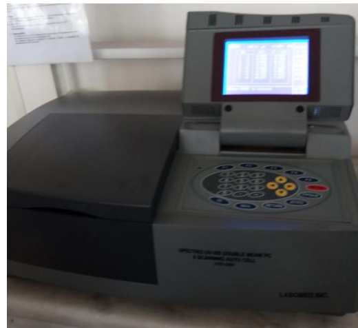
Pic G.8. Reading absorbance of sugar on spectrophotometry
