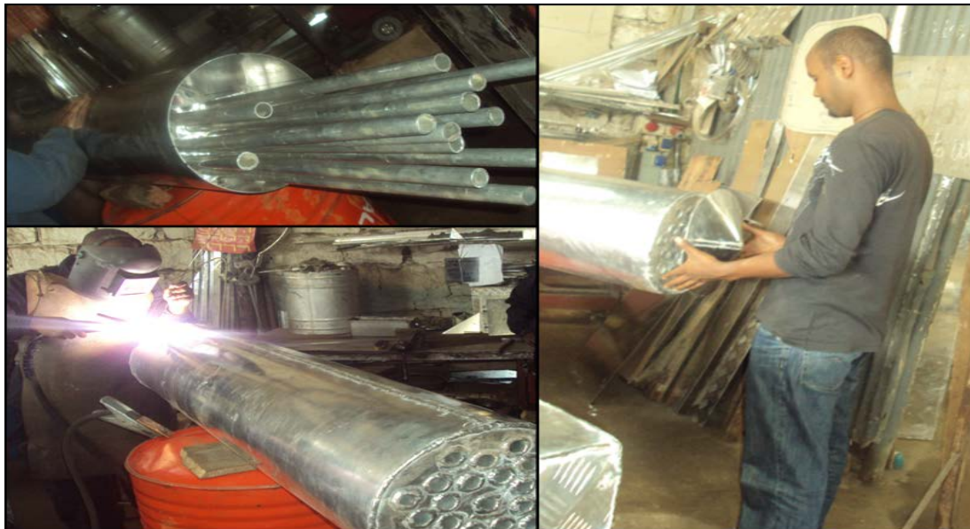
Figure 3.14 Heat exchanger manufacturing
