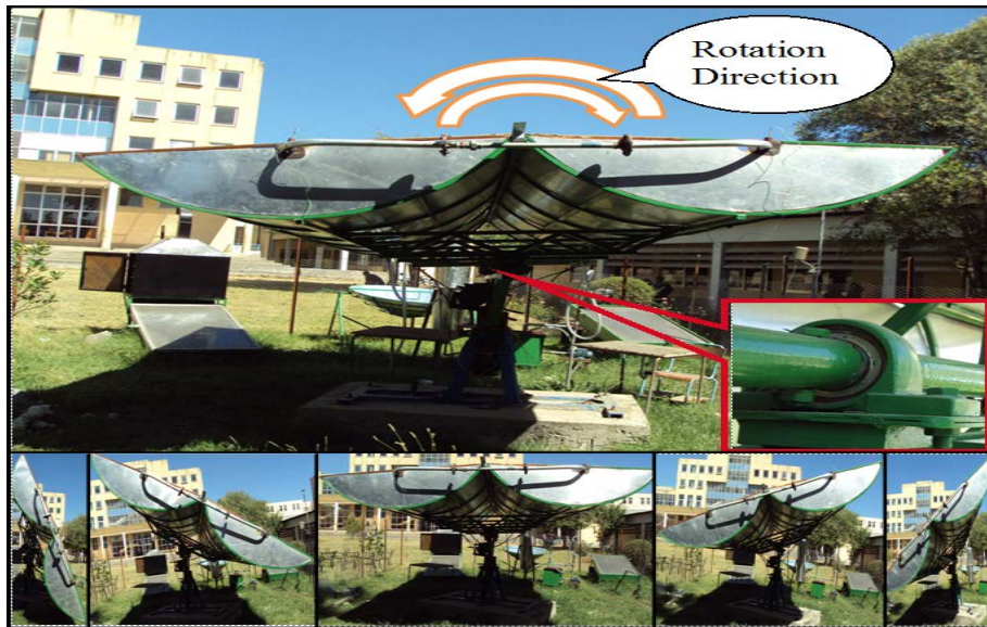
Figure 3.23 Rotational directions from east to west
