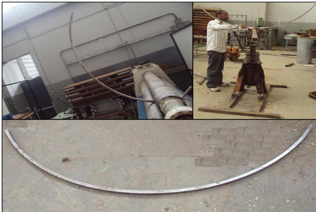
Figure 3.6 Rolling the metal frame in to parabola curve
