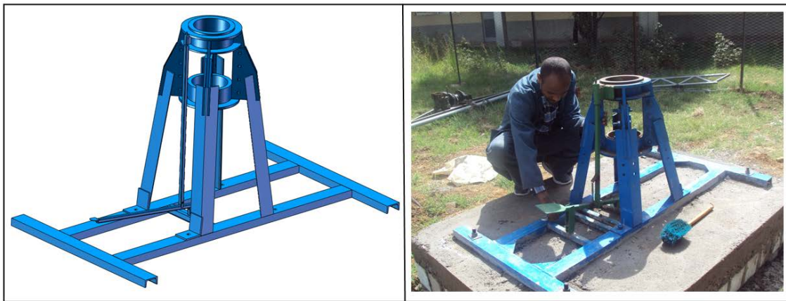
Figure 3.1 Stand of the parabolic trough
