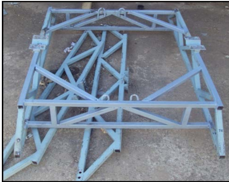
Figure 3.9 Connecting structure of the two parabolic troughs
