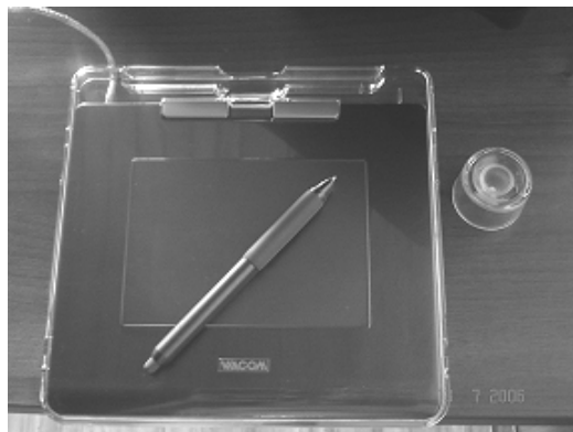
Figure 5.2 The Wacom digitizer tablet used for the data collection (model CTE-440 / Graphire 4 A7)
