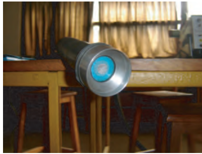
Figure 3.4: The Air Sampling Head assembled
