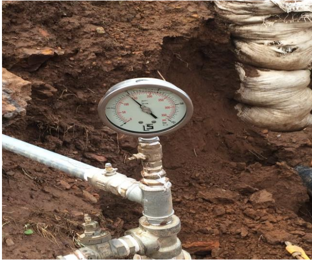
Pressure measurement by using manometer at Remera (REMEJU84)
