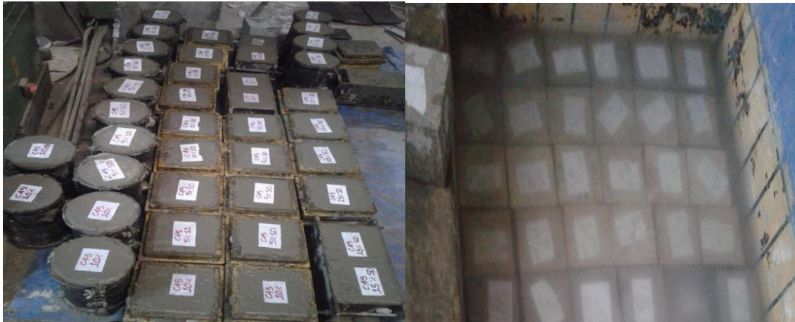
Figure 3- 8: Concrete casting and curing the samples
