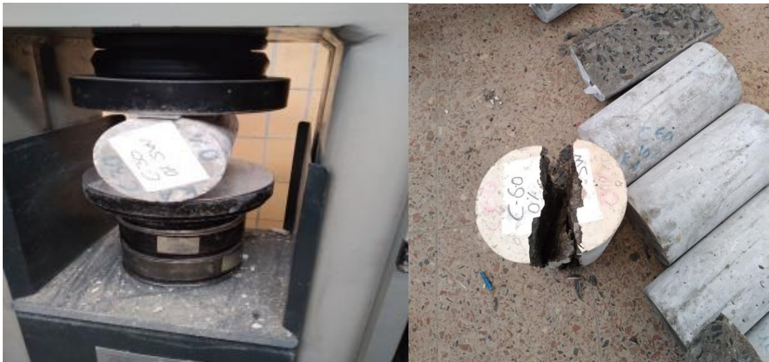
Figure 3- 10: Splitting tensile testing setup
