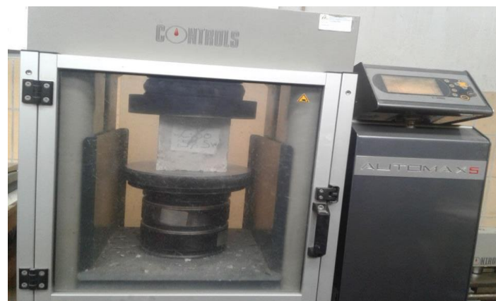
Figure 3- 9: Compressive strength test setup
