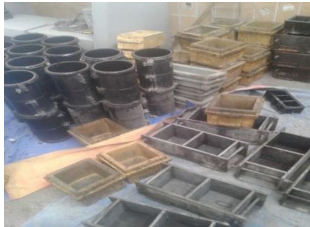
Figure 3- 6: Cube and cylinder molds for casting sealed by wax
