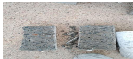
Split tensile test
