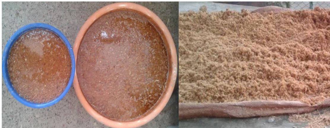
Figure 3- 5: Soaking the sawdust for 24 hours and Saturated surface drying the sawdust
