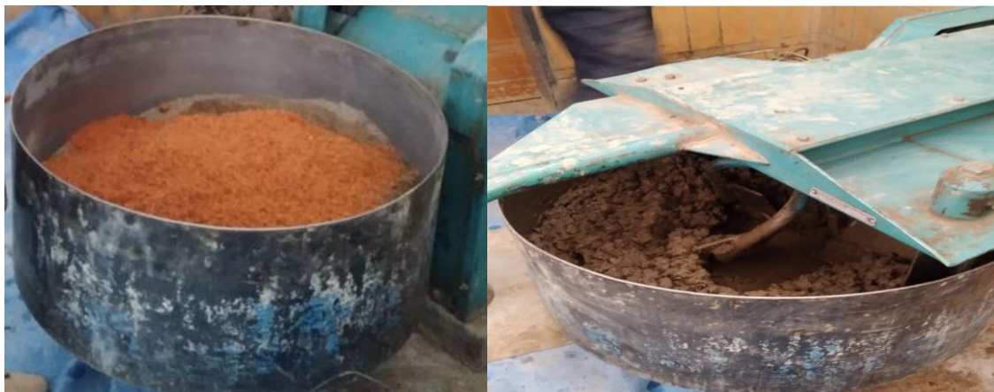
Figure 3- 7: The mixer used and mixing the concrete
