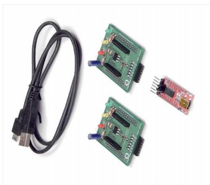
figure 21 Xbee adapter kit for the base station [66].
