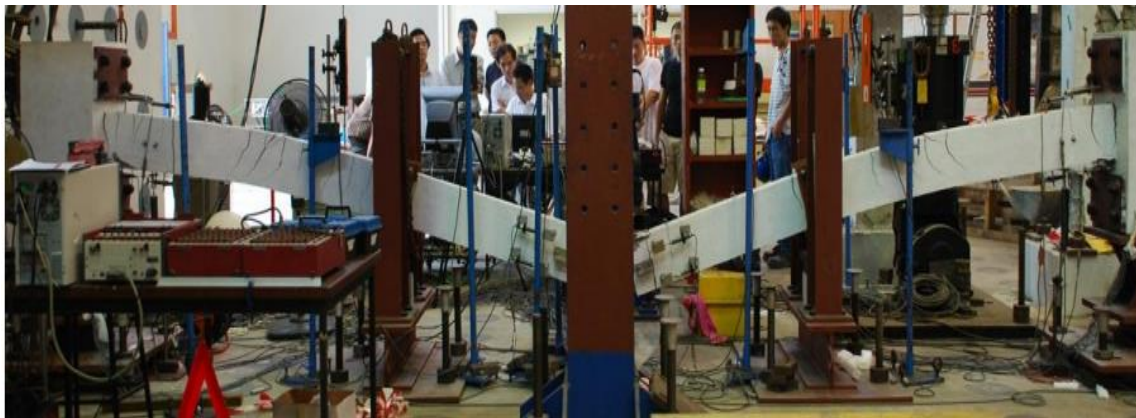
Figure 2.9: The collapse mode of the specimen (Yu and Tan, 2013)
