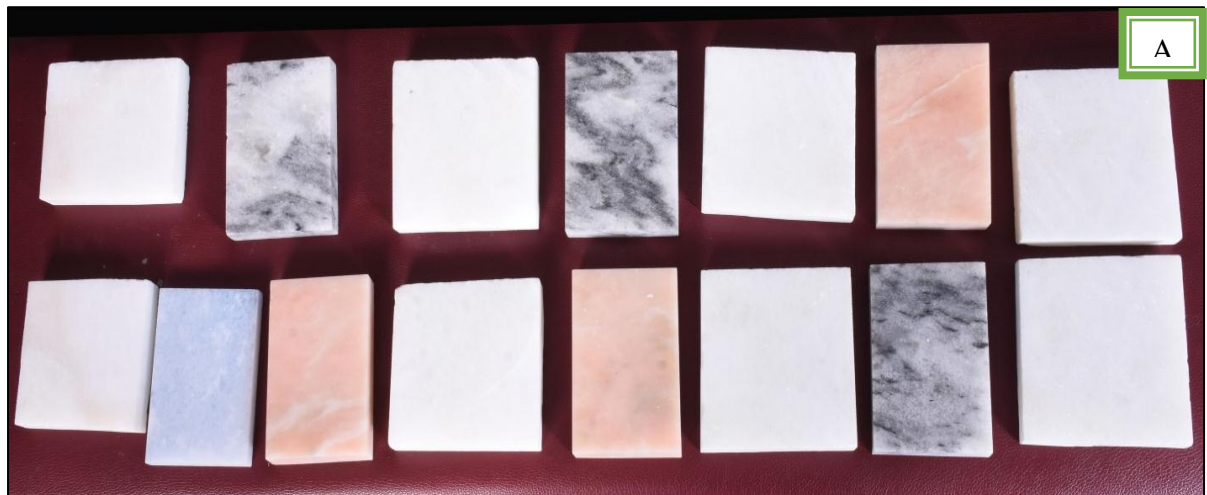
Figure 5.14: Photo, shows cut and polish sections of calcite marble samples, found in Daleti quarry with different colour.
