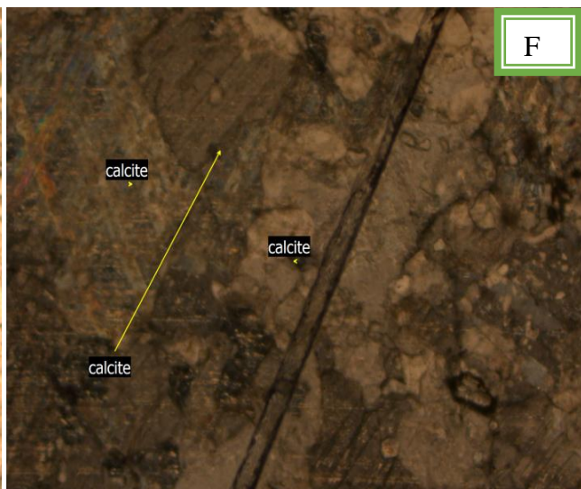
Figure 4.6: Micro-photo picture of BMC marble; sample number 04 in PPL (left) and XPL (right) in 2px magnification, show calcite is the dominant mineral.
