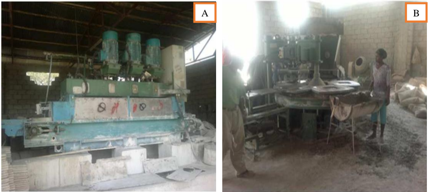
Figure5.7: A, shows, agglomerate polishing line on the left and B, Agglomerates pressing machine on the right side of the picture.
