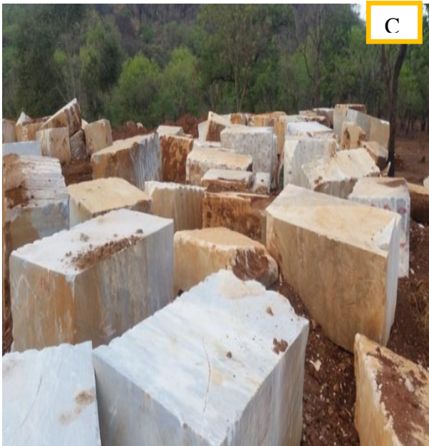
Figure 5.6: photo above:shows that, Quarry in Daleti marble where huge blocks are extracted using diamond chain saws.
