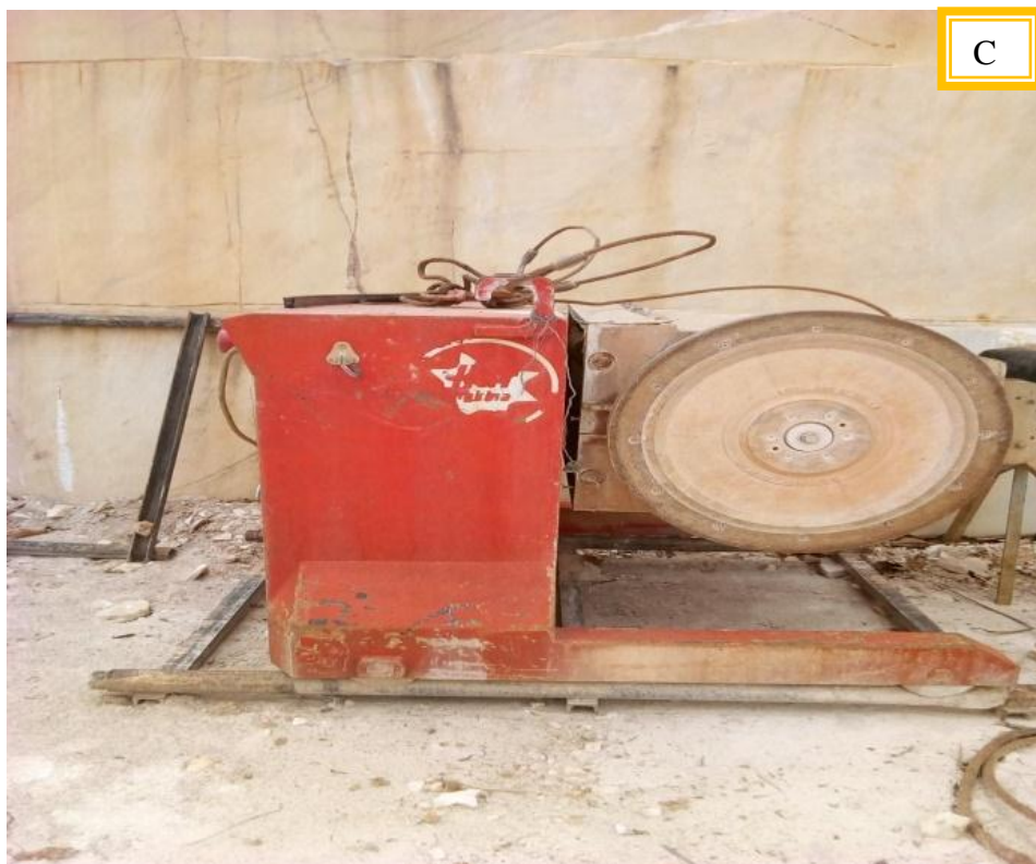
Figure 5.4: C Diamond wire saw used in cutting stone in Daleti marble quarry.
