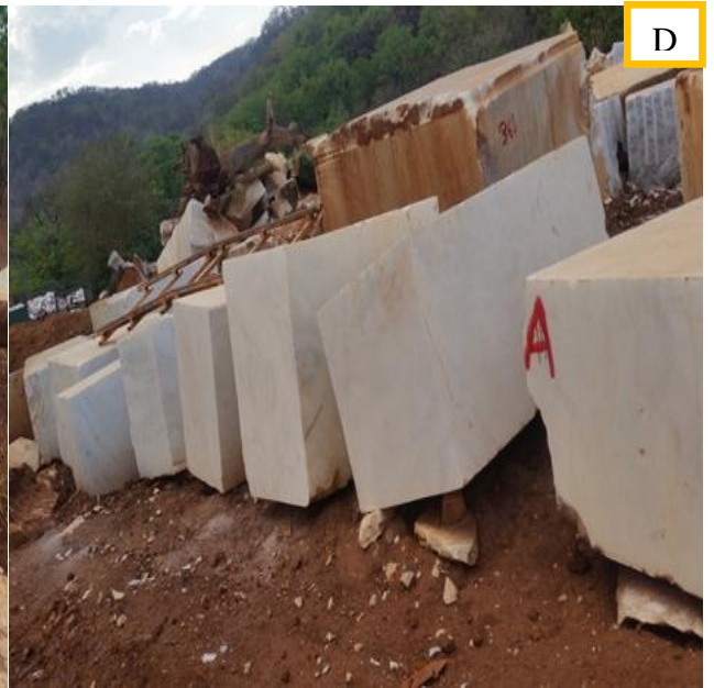
Figure 5.6: photo above:shows that, Quarry in Daleti marble where huge blocks are extracted using diamond chain saws.
