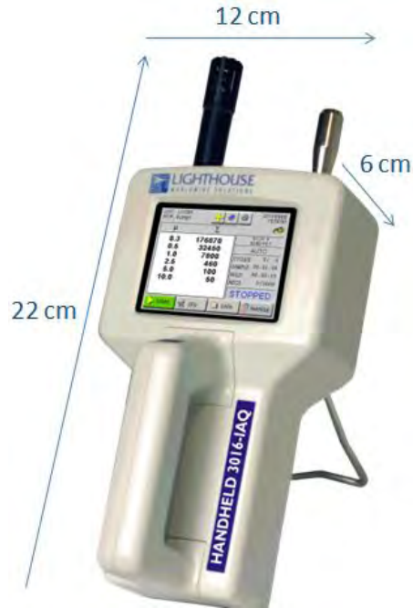
Figure 5.3: Lighthouse handheld 3016-IAQ particle counter adapted from the manual of a Lighthouse Handheld 3016 IAQ [205].
