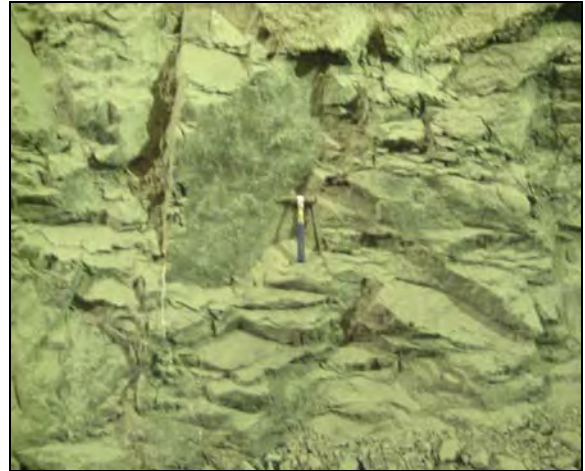
Aphanitic basalt having more than 3 joint sets and smooth joint surface
