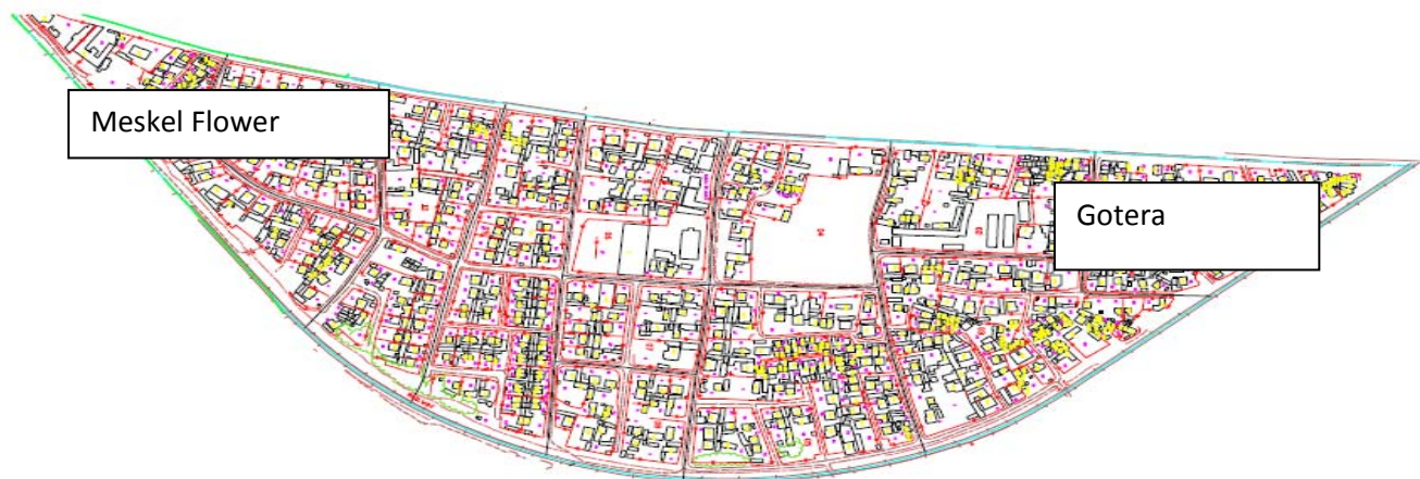
Figure 3.2 Sub-system water distributions Network
