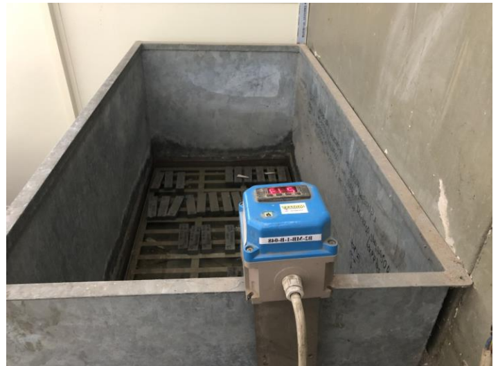
Samples at Curing tank
