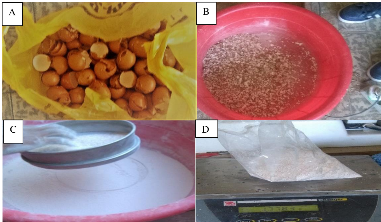
Figure 3-1. Collection & processing of egg shell, (a) raw egg shell, (b) washing & dyeing, (c) grinding & sieving, (d) measuring
