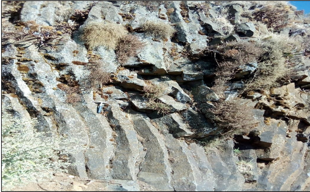
Figure 3.25: Close up view of systematic sub-vertical joints from aphyric -ophitic basalt flow (E-0497944, N-1278551, and Z-2695) having with two column faces and the rock is highly subjected by algal weathering.
