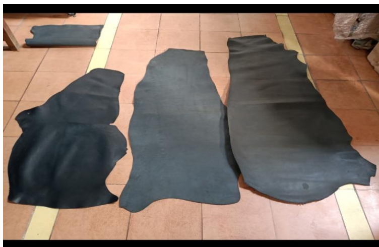
Fig 4.2 Trial 4 (IIX2), (WCTT IXZi) & Conventional chrome (IZ) respectively (the two at right end are conventional post tanned)
