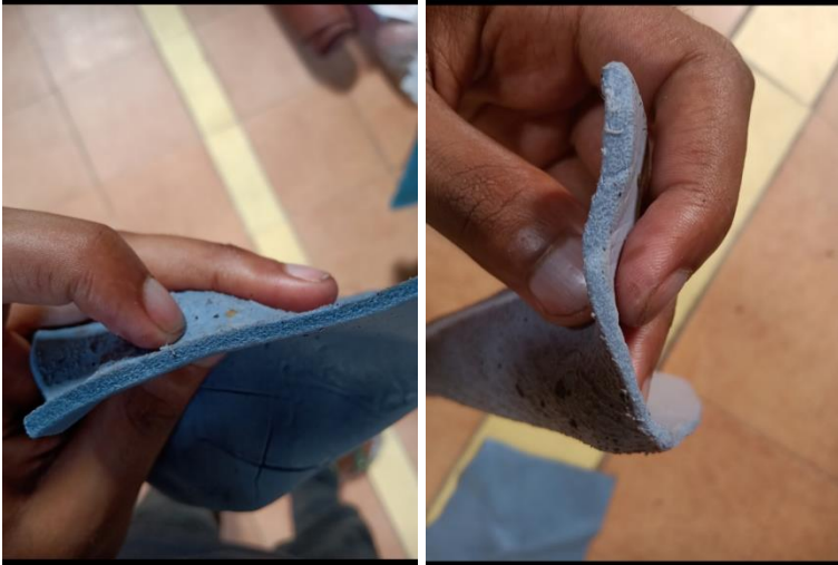
Wet blue Cross section WCTT (left) and conventional chrome tanned (right)
