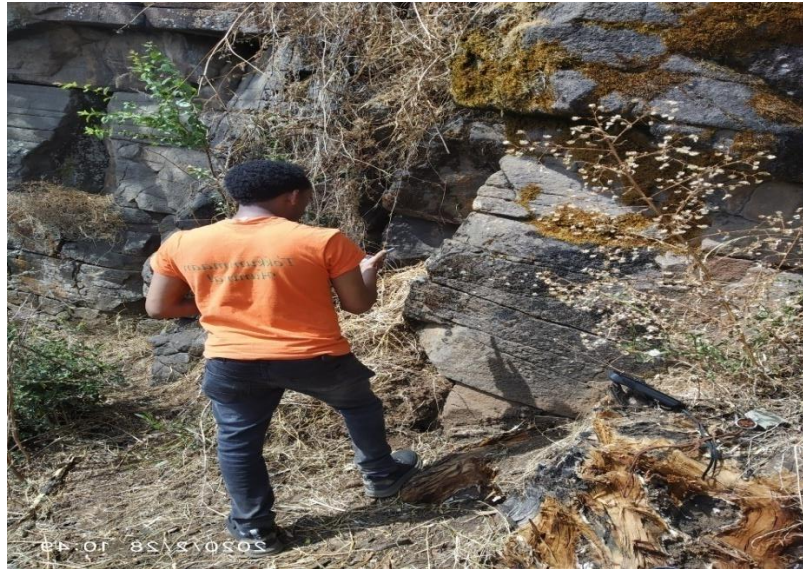
Figure 5.3 Jointed and weathered basaltic unit at top ridge of left abutment
