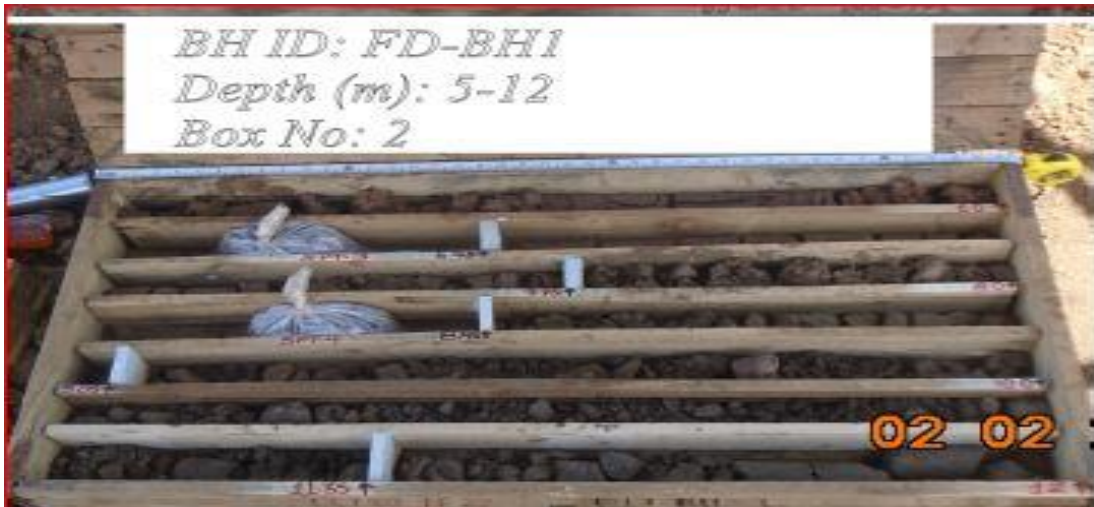
Figure 5.9 of core box shows that fractured vesicular basalt from left abutment (FDBH1)
