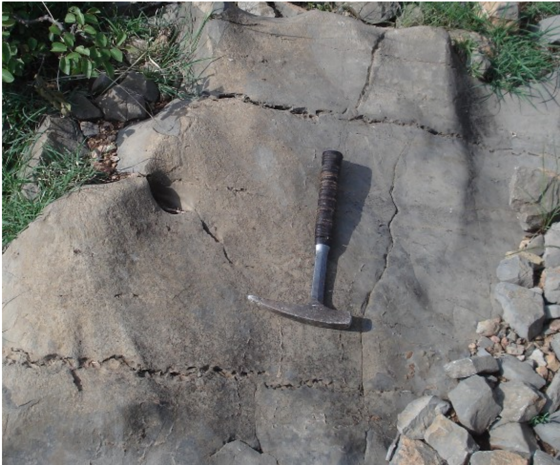
Figure 5.2. Multi-macro-stylolites at out crop level, on the exposed micritic limestone. Field photo taken at Dachatu river section, Dire Dawa area.
