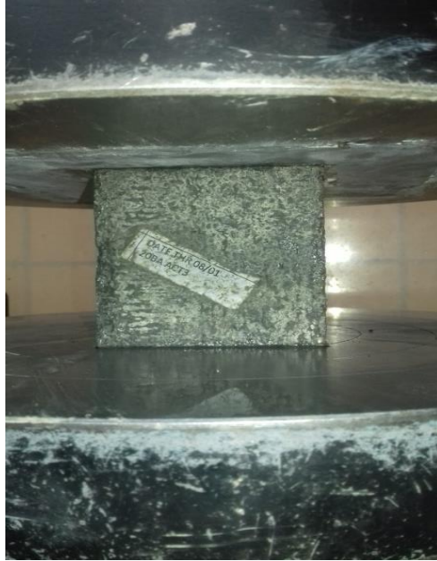
Figure 4.5 Compressive strength test for mortar cube
