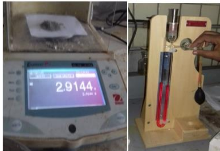
Figure 3.1 Determination of fineness by blain air apparatus
