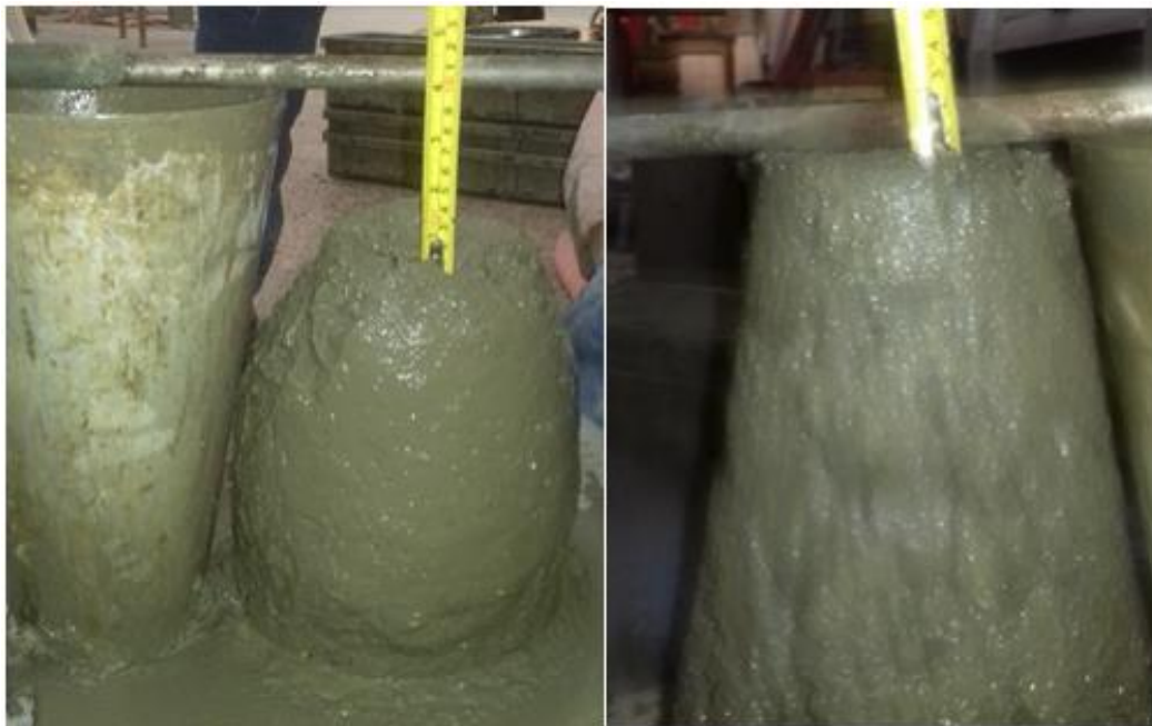
Figure 4.3 Slump of the control concrete and 30%BA concrete
