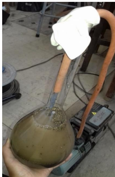
Figure 3.2 Specific gravity test for fine aggregate
