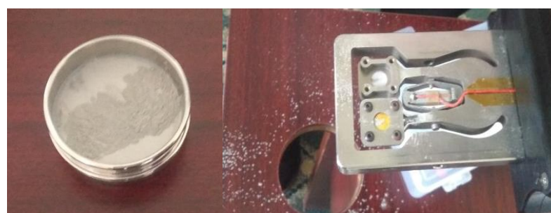
Figure 4.7 Xrd test of grounded hydrated cement
