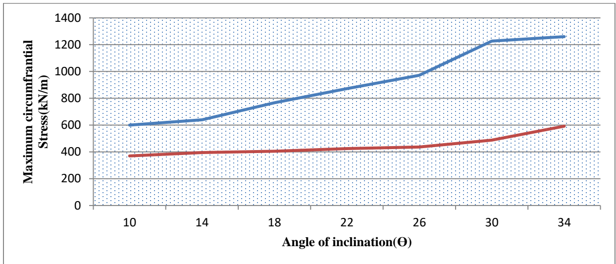
Figure 4 25 Shell stress of corrugated barrels with variable Angle of inclination
