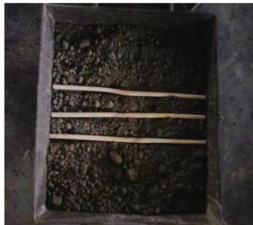
Figure 14:Top view of placement of reinforcement and sample preparation
