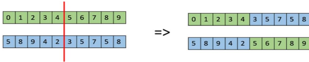
Figure 3.9: Diagram representation of one-point crossover.
