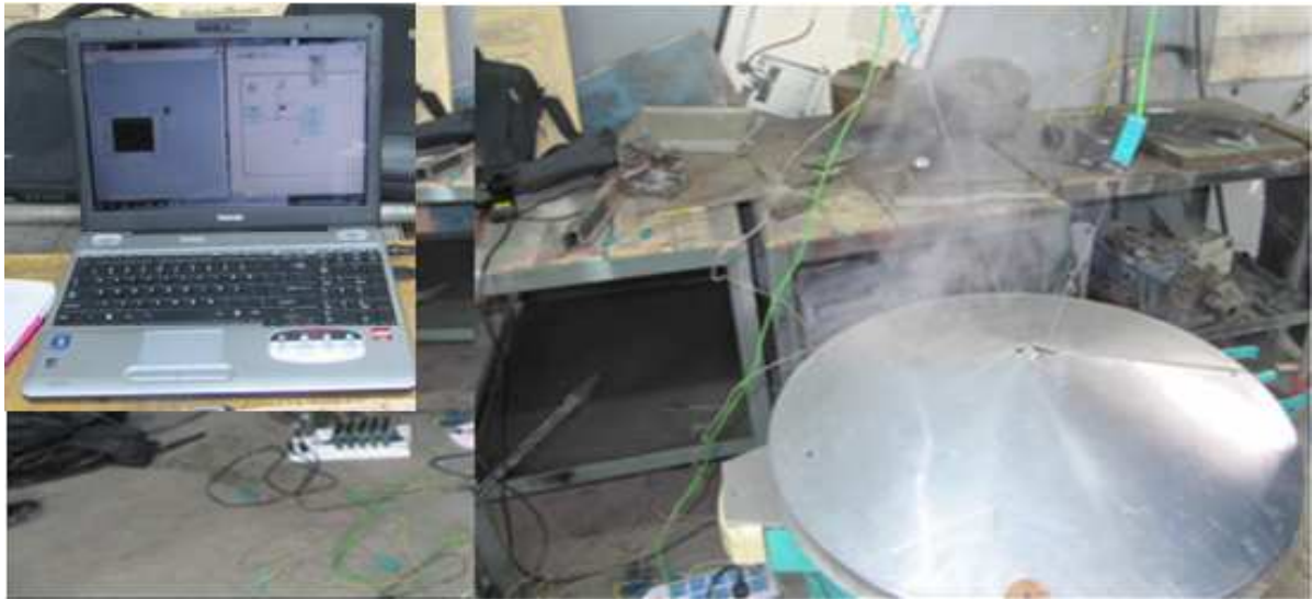
Figure 4-1: Experimental set up to measure heat up time.
