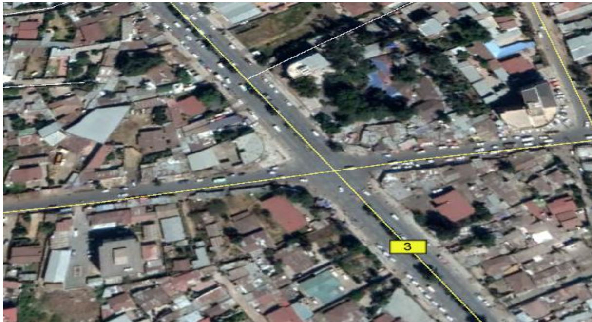
Figure 3.5 Semein Mazagjah Two-Way Stop Controlled Intersection
