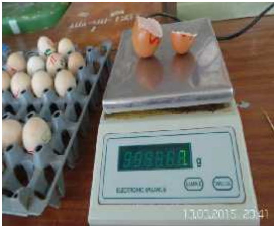
Weighing egg shell by using digital balance
