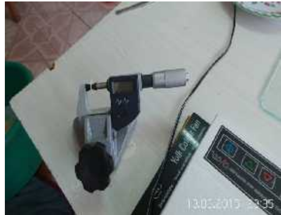
measuring shell thickness by using digital caliper
