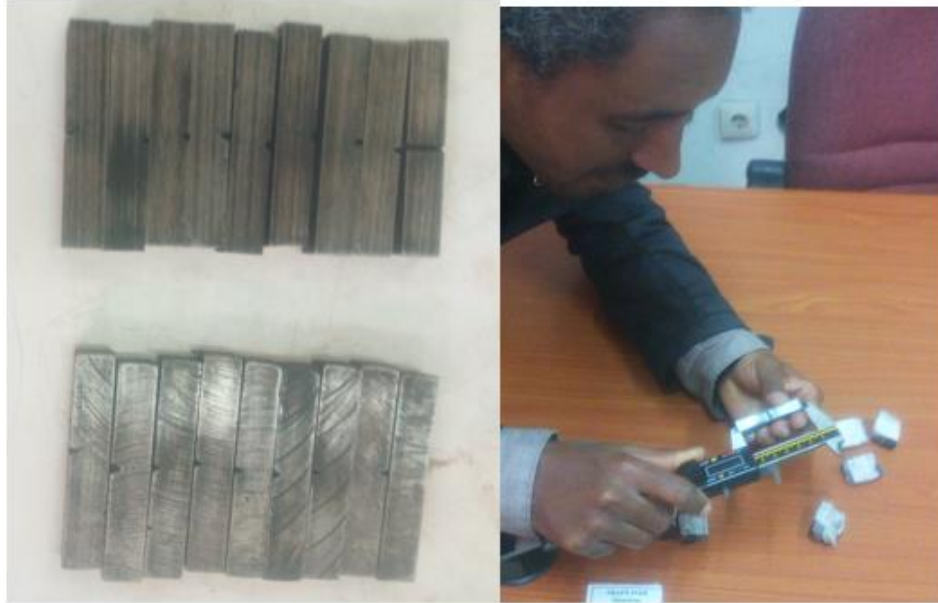
Figure 3.9 checking prepared specimen dimension for impact test
