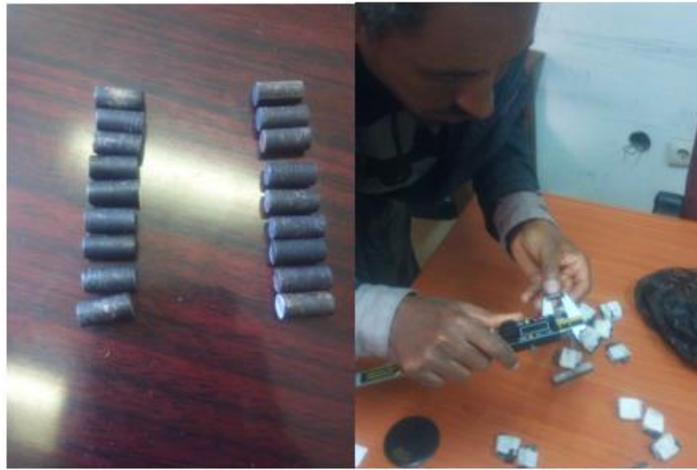
Figure 3.13 checking prepared specimen dimension for wear test
