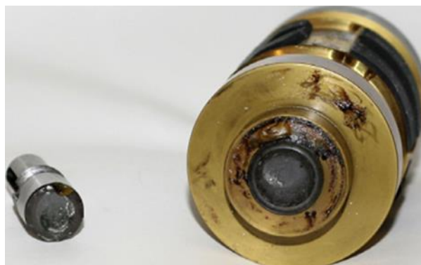
Figure.2.2 Fractured Parts of the Die
