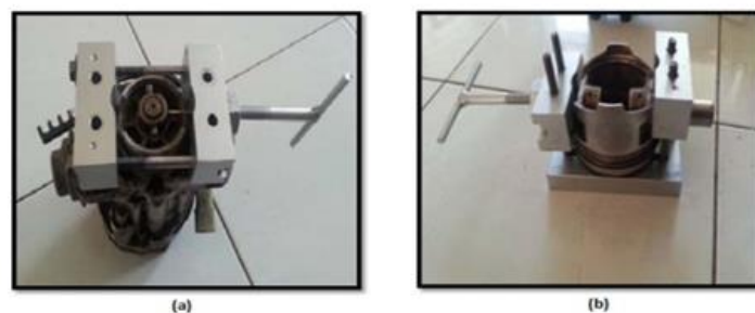
Fig. 2.1 (a) Process removal distributor pin using a jig. (b) Process removal piston pin using a jig and fixtures [43]
