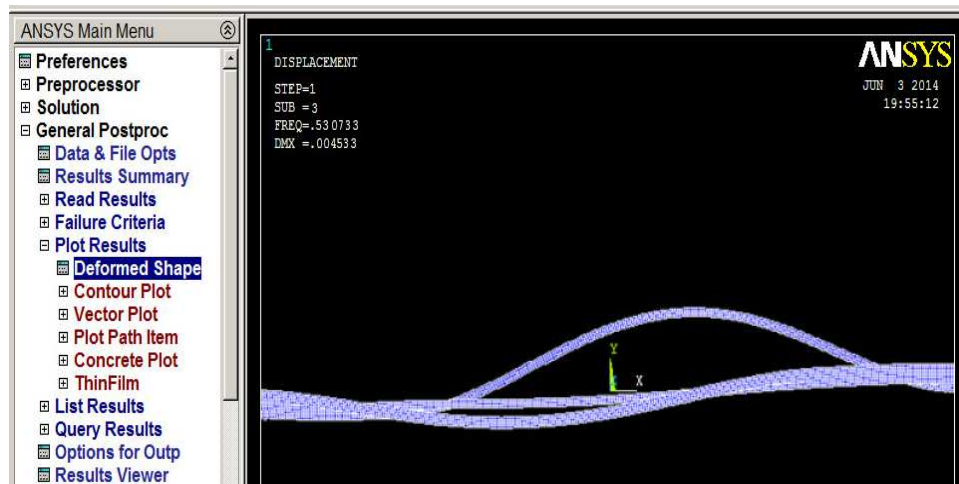
Figure 4.37 d) Third mode of double centered delamination clamped-clamped beam with zoom in
