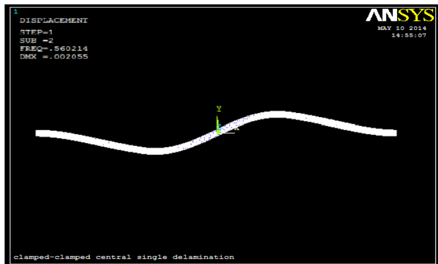
Figure 4.25- Second mode of single centered delamination clamped-clamped beam
