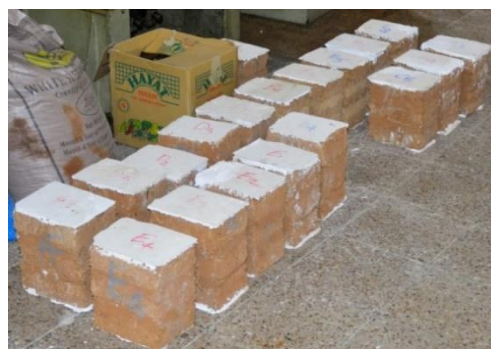
Figure 4-8 Prisms capped ready for Compression Test
