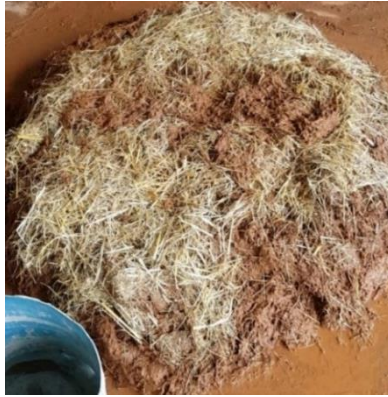
Figure 4-4 mud composed of sand silt clay and straw
