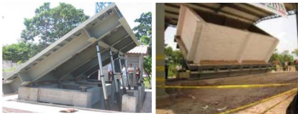
a) Tilt table with 40 degrees as maximum angle b) reinforced wall tilted
