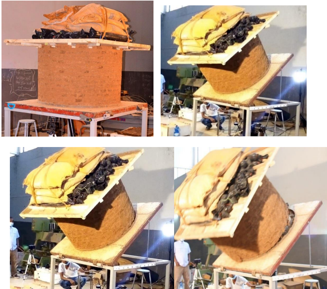
Figure C-4 4 th Case loading tilting the circular adobe model with an addition of load and no crack is seen but the toe detaching is observed
