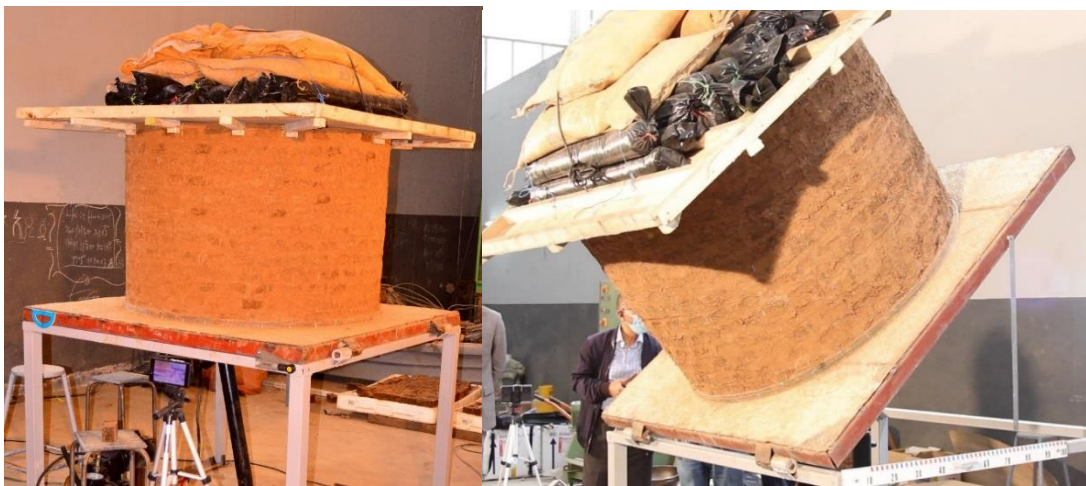
Figure C-2 2 nd case loading tilting the circular adobe model
