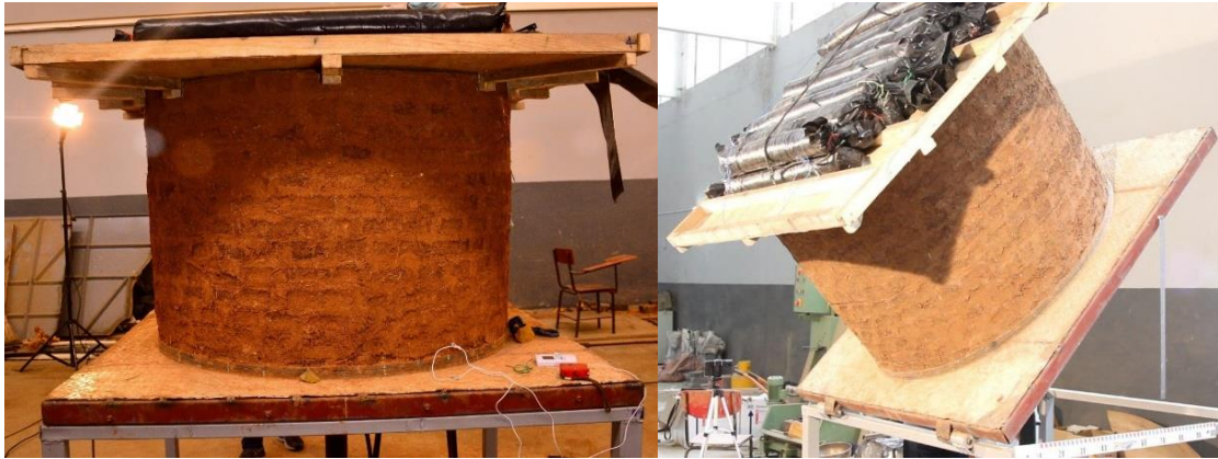
Figure C-1 1 st Case loading tilting the circular adobe model
