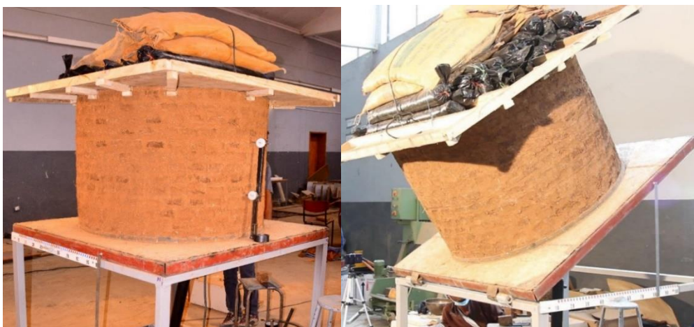
Figure C-3 3 rd Case tilting the circular adobe model with an addition of load and no crack is seen
