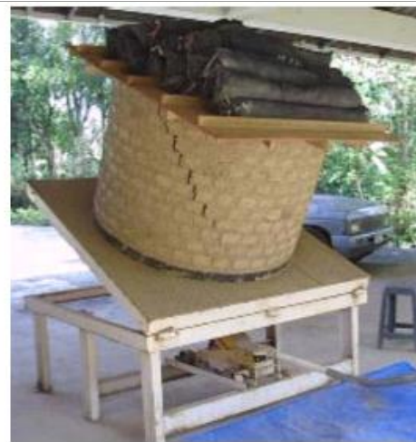
Figure 2-9 Tilting the specimen until cracking and subsequent failure (Jinwuth 2012)
