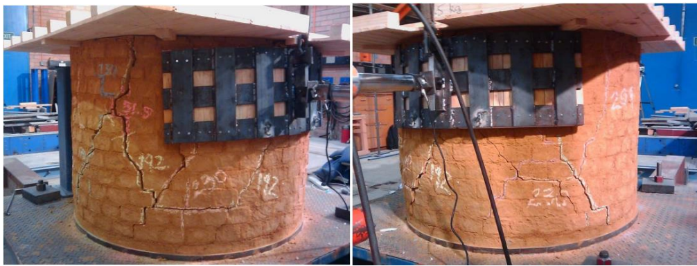
Figure 2-10 Failure crack patterns at the southwest and southeast side wall (Jinwuth 2012)
