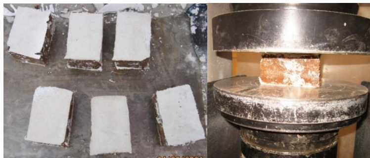
Figure 4-18 capping and testing of the reduced scale unit adobe
