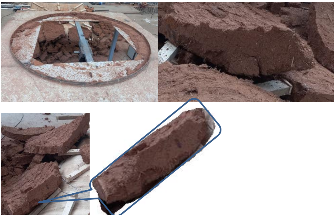
Figure C-5 the model after the base detached
