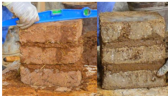
Figure 4-7 construction of the adobe prism
