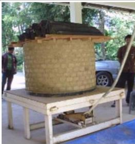
Figure 2-9 Tilting the specimen until cracking and subsequent failure (Jinwuth 2012)
