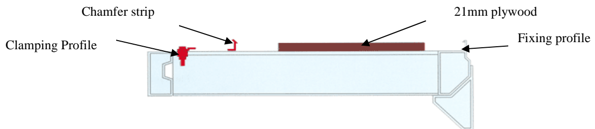
Figure 3.12 PERI RAPID clamping principle
