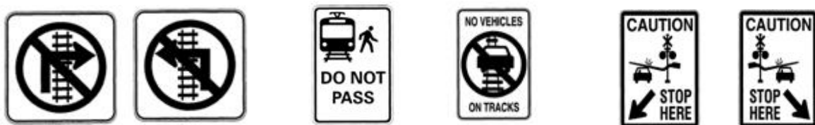
Figure 2.6: No Turn Sign, Do Not Pass Sign, No Vehicles On Tracks Sign, and Stop Here Sign
