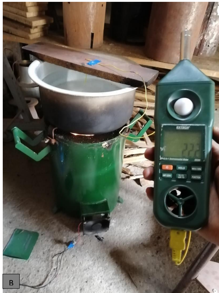
Figure 3.11 (a) schematic of the experimental setup (b) actual experimental set up of microgasifier stove
