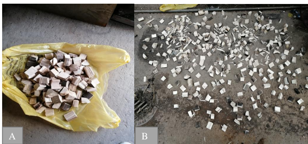
Figure 3.1(a) Eucalyptus wood sized for usage, (b) sun-drying of the wood fuel
