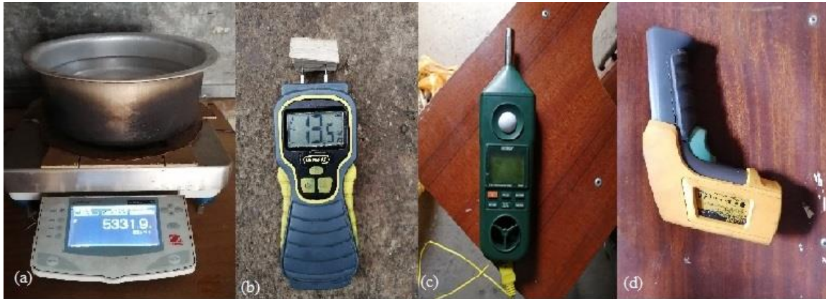
Figure 3.2 Equipment used: (a) platform balance, (b) wood moisture meter, (c) environmental meter, (d) infrared thermometer
