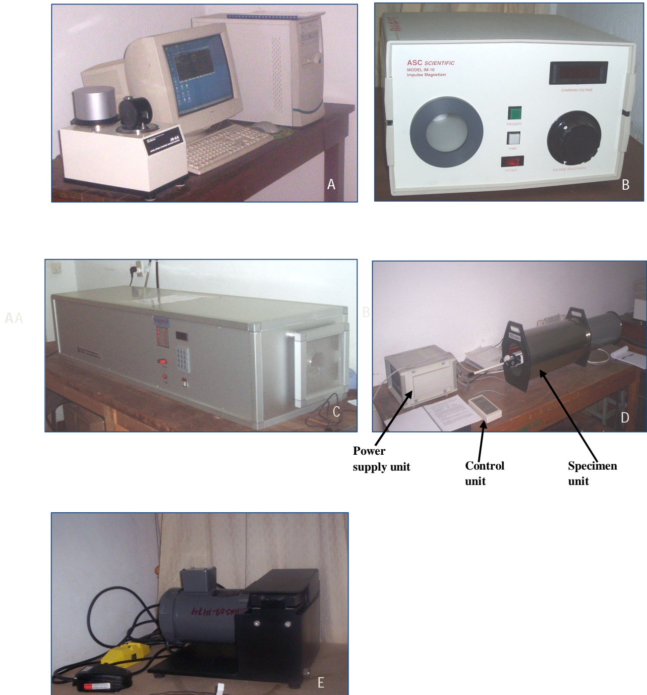
Fig.5.2. Laboratory facilities for Paleomagnetic study in Earth Sciences dept. of AAU .A) JR-6A spinner magnetometer attached to Dell machine; B) ASC Impulse Magnetizer; C) MMTD Thermal demagnetizer; D) LDA-3A Alternating filed demagnetizer; E) Dual blade core slicing saw.
