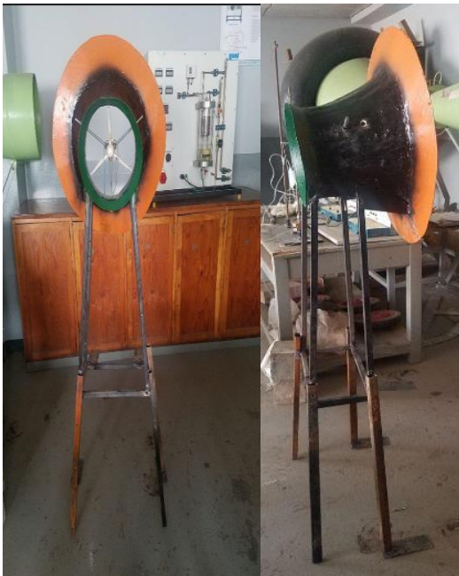
Figure 6.2 Different views of the model of brim diffuser with stand
