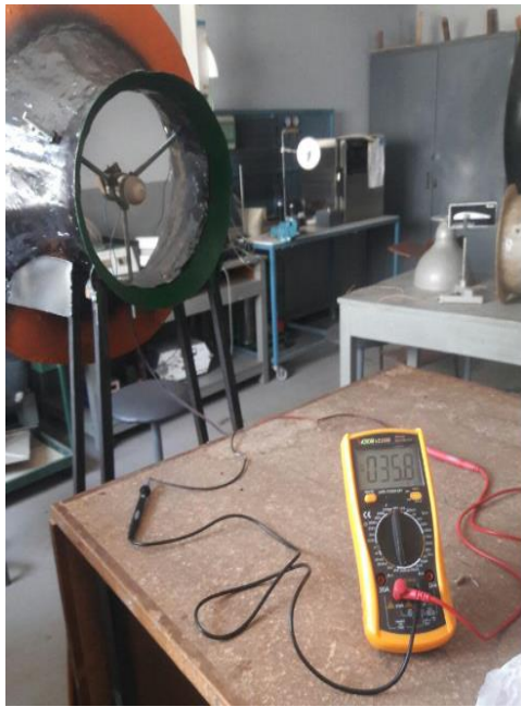
Figure 6.10 Multimeter connected in series with load to measure current flowing through it and its electrical circuit
