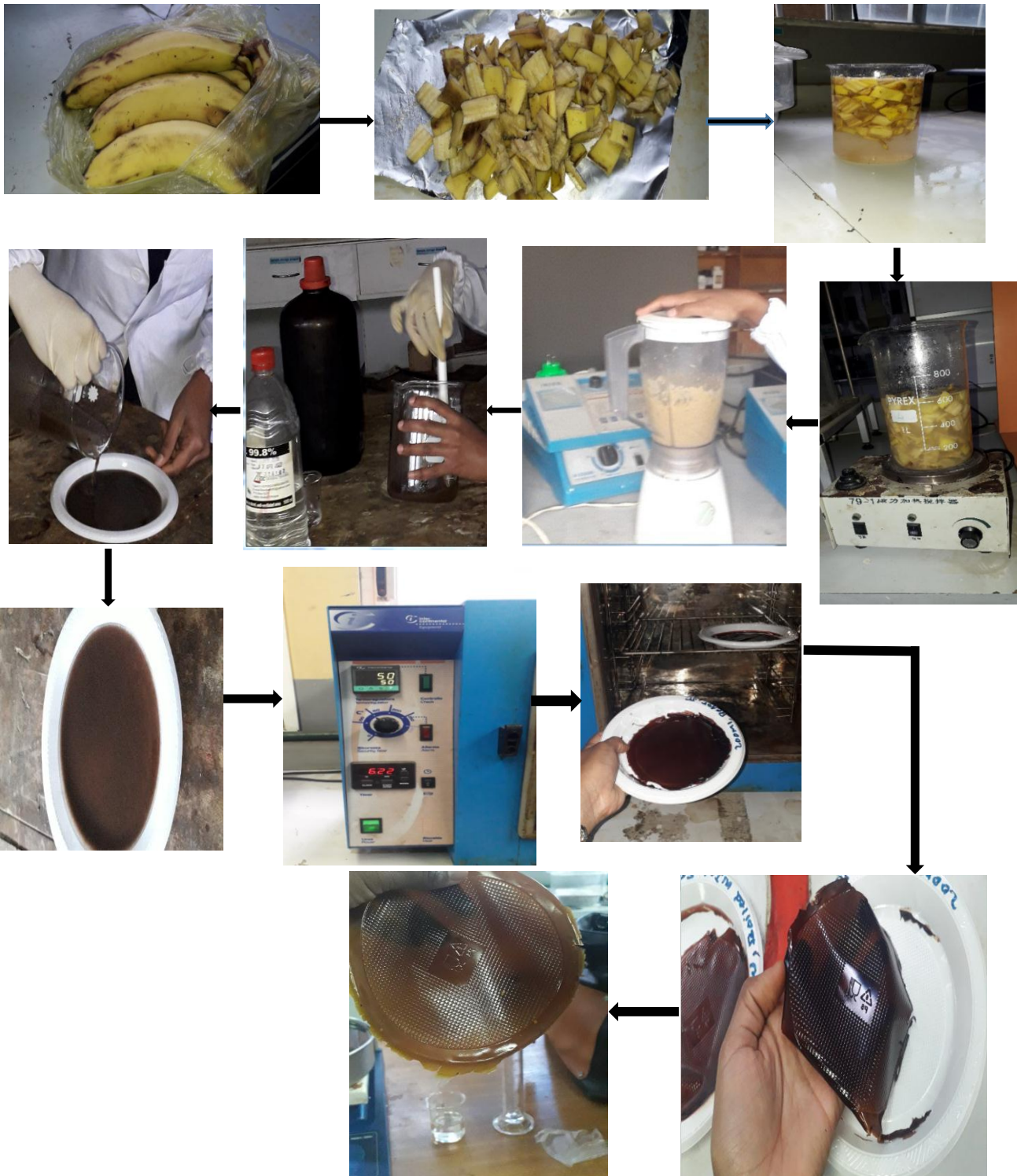
Figure 3-2: Banana peel based bio plastic synthesizing procedure
