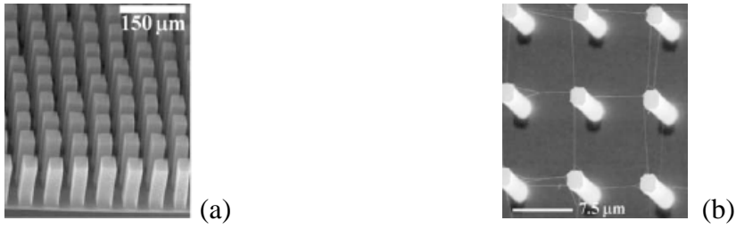
Figure 30. a) Structured pattern of SiO 2 on Si wafer b) Directed growth of CNTs [33]
