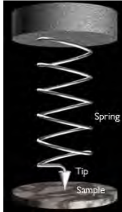
Fig.41.Schematic illustration of the AFM with a tip attached to a spring
