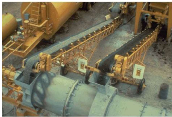
Figure 2-2: Hot recycling utilizes the heat-transfer method
