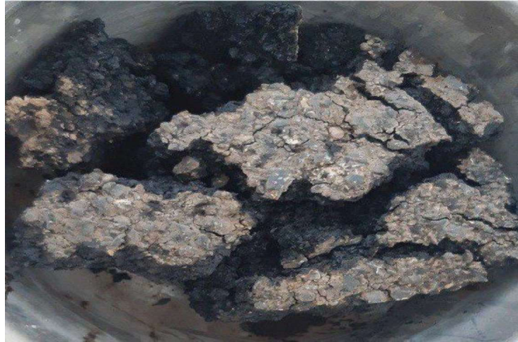
Figure 3-2: Sampling RAP from the stockpile
