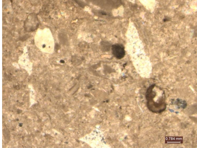
Figure 4.2: Photo Optical microscopes of moldic pores. Samples from Calub Core No. 4, 2228m.
