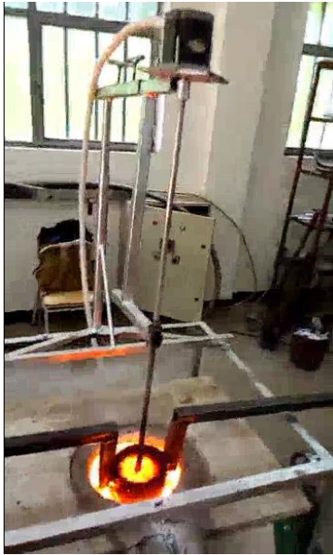
(a) Mixing of Al6061 TiB 2 by stirrer (b) Adding the molten MMC to mold (c) cooling the MMC
