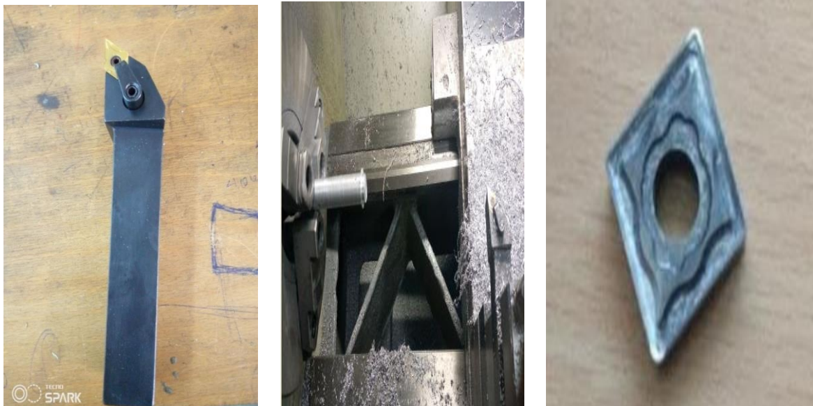
(a) Carbide cutting tool (b) Carbide cutting tool in CNC lathe machine (c) Tool bit
